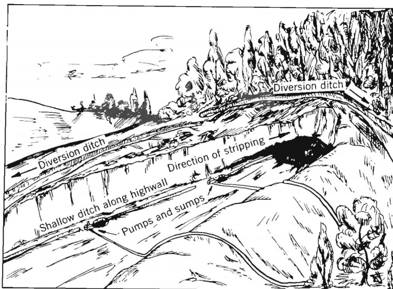
FIGURE 11. - Sketch of Strip Mine Drainage Control Measures for Surface and Ground Water.
